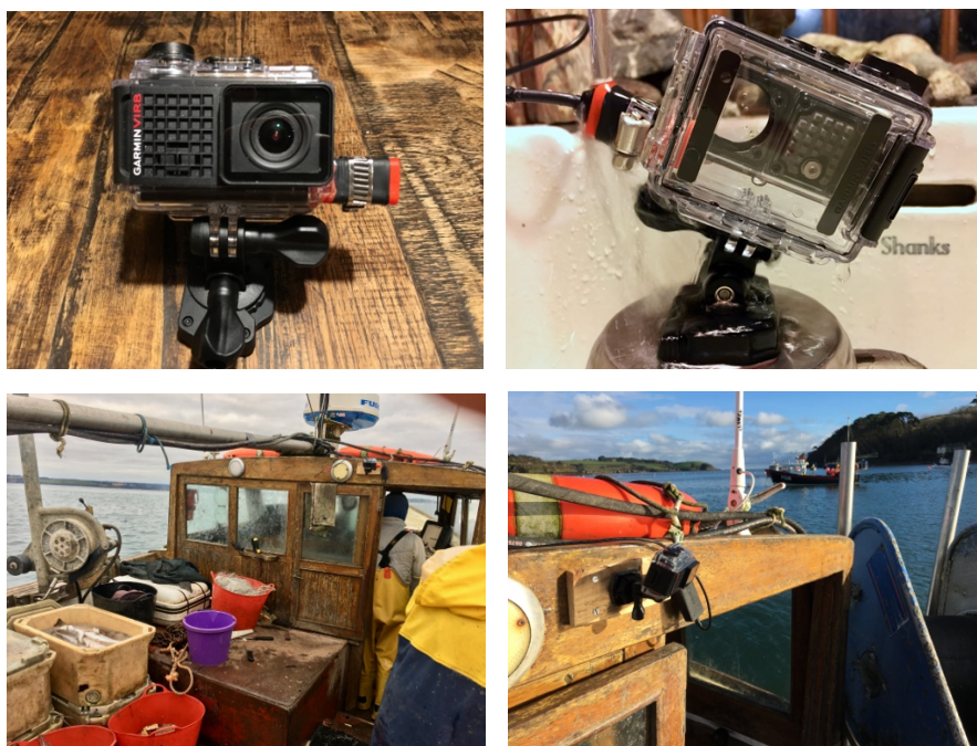
Figure 11. Garmin VIRB Ultra 30 in its waterproof housing with the custom made entry point for the vessel 12v DC power supply, complete with Jubilee clip; undergoing a 12 hour water endurance test; and two images of the camera in situ on board Lady Hamilton .
