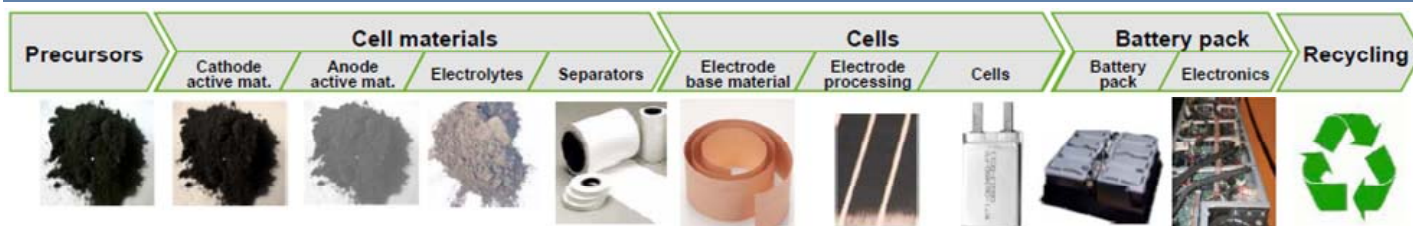
Exhibit 7.2: Lithium-ion battery manufacturing process
