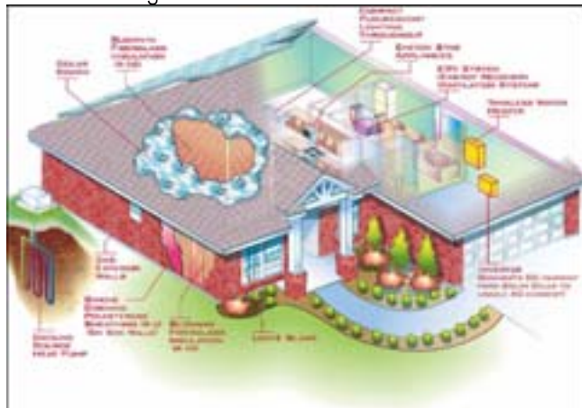
Figure 59 Schematic design for a zero carbon home
